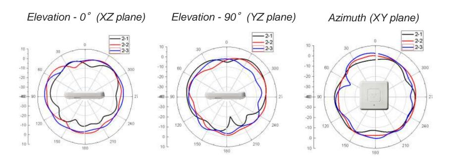
**Radiation Plots** – a general guide to tell you where most of the energy and receive sensitivity of the Cisco APs is being directed.
